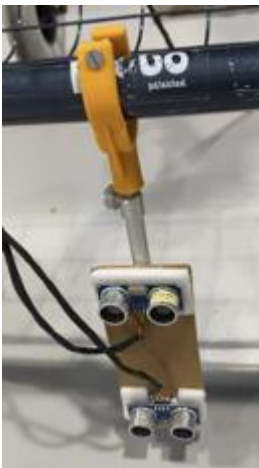
Figure 18: sensor plate attached to a walker with screw through yellow mount and sticker marking on sensors
