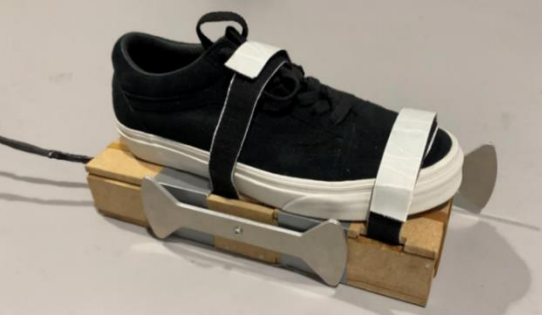
Figure 27: Box with shoe, horizontal rods and Velcro straps
