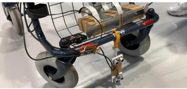
Figure 26: attached sensor plate, perfboard and battery on walker
