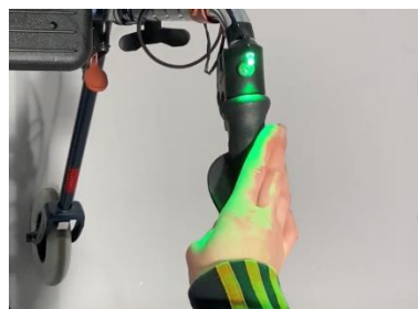
Figure 23: led placement on walker
