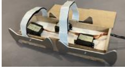
Figure 13: the box with lid off, rods, motors, Velcro straps and Styrofoam
