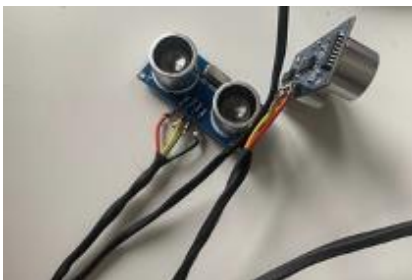
Figure 24, heat shrinking tube around wires
