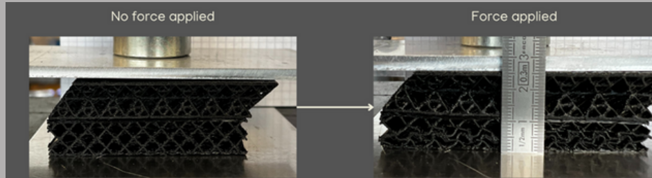
Figure 56, Sample 1 and grid structure under a hydraulic press
