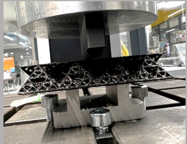
Figure 36, Photo of 3 points bend test set-up
