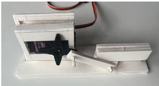
Figure 154, servo rotary to horizontal for slide out dispenser side view
