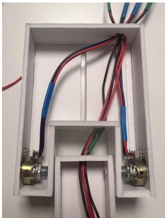
Figure 165, slider with wiring and. Potmeters
