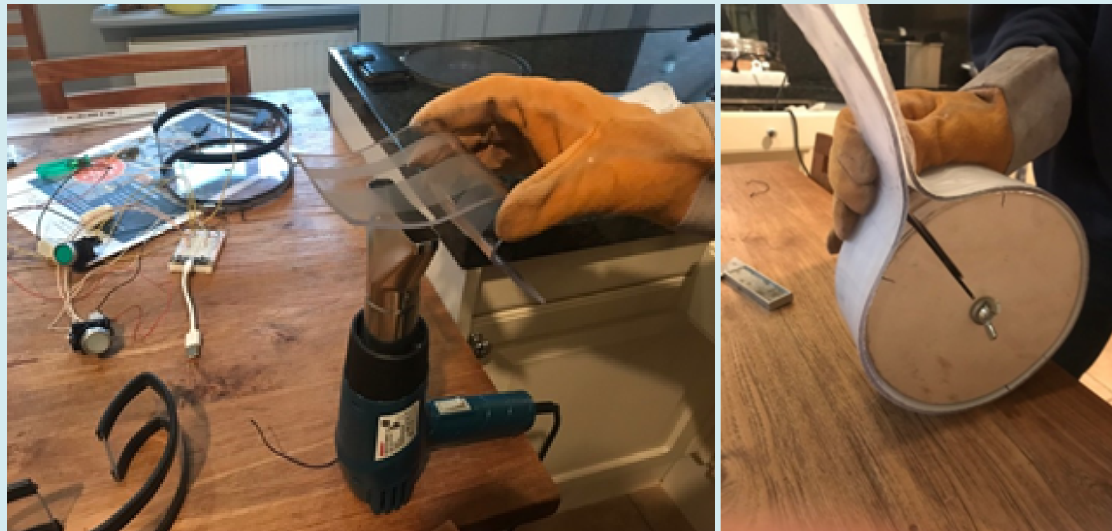
Figure 12: Bending the PVC with heat fohn for outside component.
